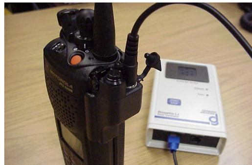
Motorola portable/BDN6676 connected to Rosetta-Lt with 034-184-023A radio cable
