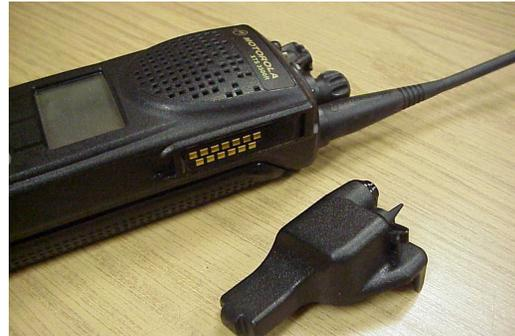
Motorola portable showing Accessory Port and BDN6676 audio adapter
