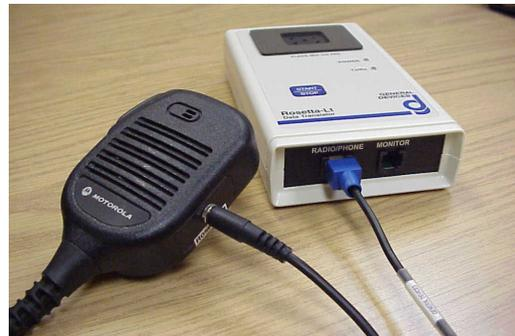
Modified Motorola Spk/Mic connected to Rosetta-Lt with 034-184-023A radio cable
