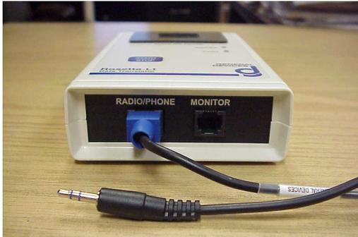
Rosetta-Lt with 034-184-023A radio cable (commonly used with radio adapters)
