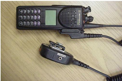
Motorola portable with Spk/Mic (modified to add a Rosetta jack)
