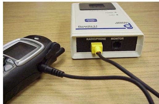
Cell phone connected to Rosetta-Lt with 034-184-022A cell phone cable
