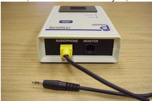
Rosetta-Lt with 034-184-022A cell phone cable (commonly used with cell phone headset jack)
