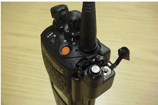
Motorola portable with BDN6676 audio adapter
