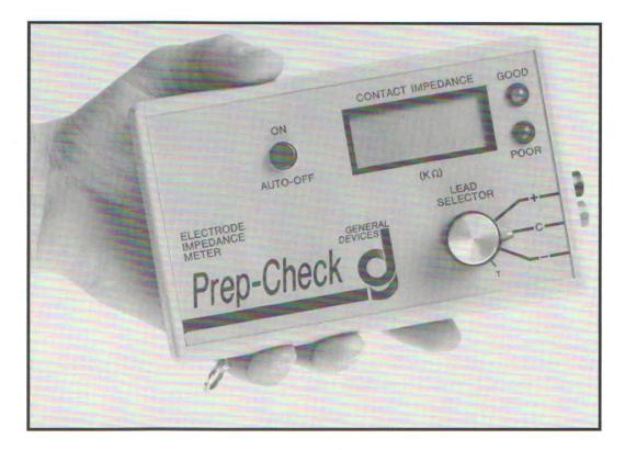
General Devices' Prep-Check Electrode Impedance Meter improves quality of biopotential monitoring by fast, simple, and accurate assessment of lead wires, electrodes, and electrode site preparation. Ideal for physicians, nurses, and technicians applying electrodes for ECG, Holter, Stress Testing, EEG, EMG, Evoked Response and other bio-potential measurements. Perfect as teaching aid and for sales demonstrations.
