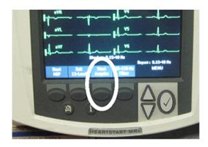
3. To send the 12-Lead to Rosetta-DS, press the Menu button and select Send.
